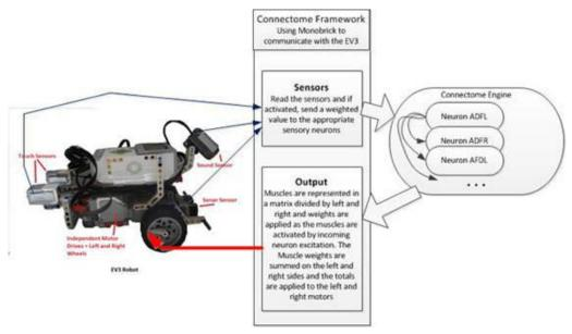
The software works with sensors and effectors provided by a simple LEGO robot. The sensors are sampled every 100ms. For example, the sonar sensor on the robot is wired as the worm's nose. If anything comes within 20cm of the "nose" then UDP packets are sent to the sensory neurons in the network. The same idea is applied to the 95 motor neurons but these are mapped from the two rows of muscles on the left and right to the left and right motors on the robot.
