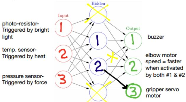
If temp and pressure sensor reach threshold, hidden layer #1 activates buzzer with a low tone (hot) and #2 activates gripper motor
