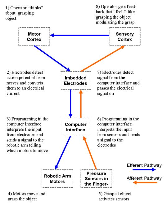
Abstraction of a closed loop BCI operated robotic arm
