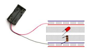
Insert one end of a wire anywhere along column of red wire from battery pack, and insert the other end of the wire in the same row as the positive end of the LED.
