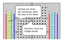
The two columns along the side are for powering the board. You will notice a (+) on one side and a (-) on the other. When connecting a battery pack, the red wire goes to (+) and the black wire goes to (-).
